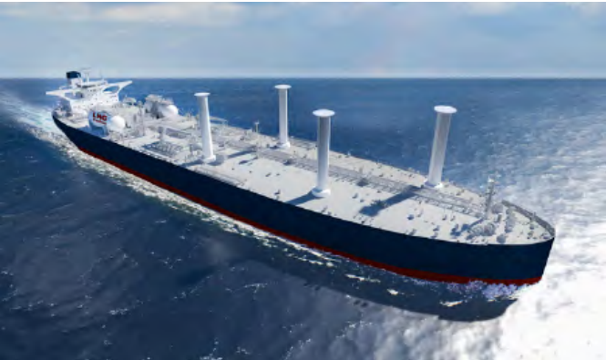
Hi-Rotor(New concept eco-friendly sail)
